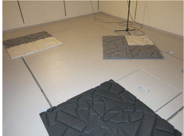
Figure B3.8: Cropfield during the measurement of sound absorption area for groups of 4 objects.
