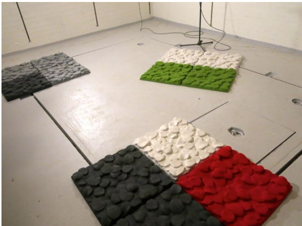
Figure B3.5: Leaves during the measurement of sound absorption area for groups of 4 objects.
