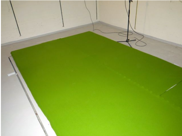
Figure B3-3: Frequency wall 80 mm during the measurement of sound absorption coefficient.
