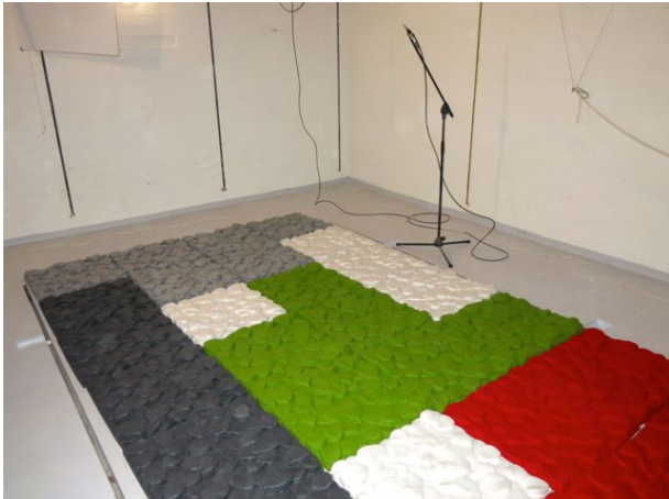
Figure B3.1: Leaves during the measurement of sound absorption coefficient.
