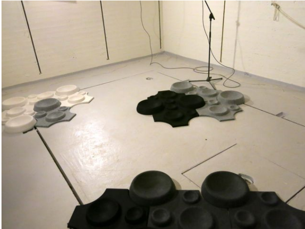
Figure B3.7: Moon during the measurement of sound absorption area for groups of 4 objects.
