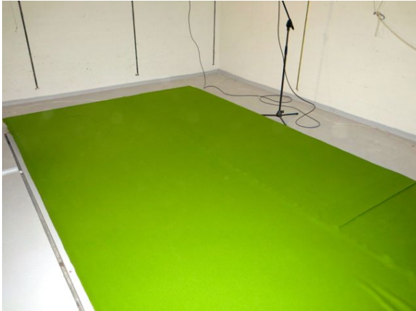
Figure B3.4: Frequency wall 120 mm during the measurement of sound absorption coefficient.
