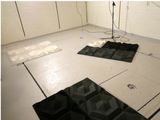
Figure B3.6: Beehive rectangular during the measurement of sound absorption area for groups of 6 objects.
