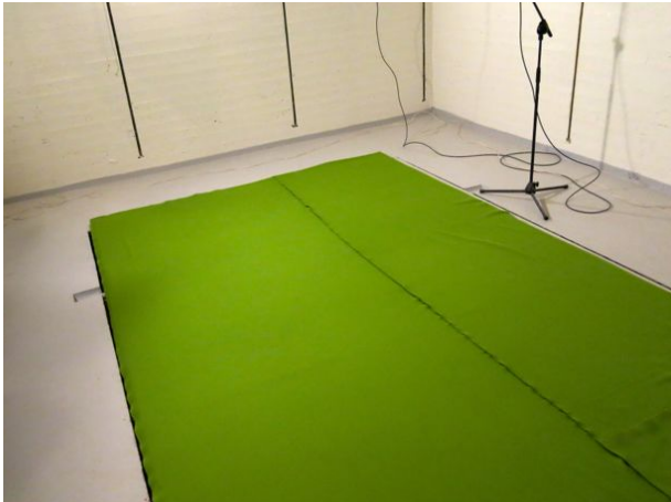
Figure B3.2: Frequency wall 40 mm during the measurement of sound absorption coefficient.
